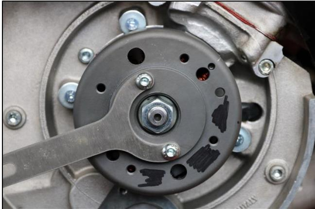
Abbildung 3 – mounted blocking bracket
