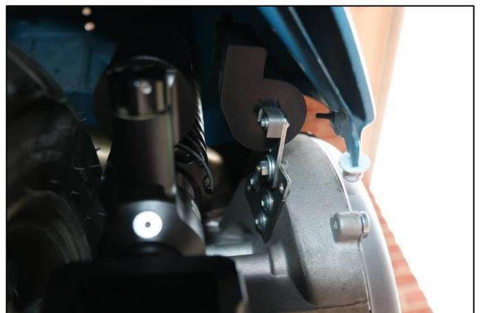
Abbildung 9 – Ignition coil, on original position
