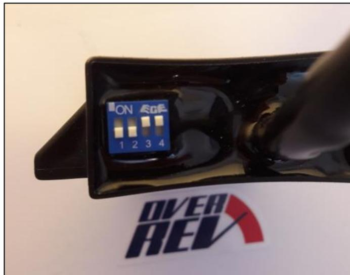
Abbildung 12 – example picture – timing curve #2 (0011)
