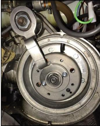
Abbildung 2 – mounted blocking bracket
