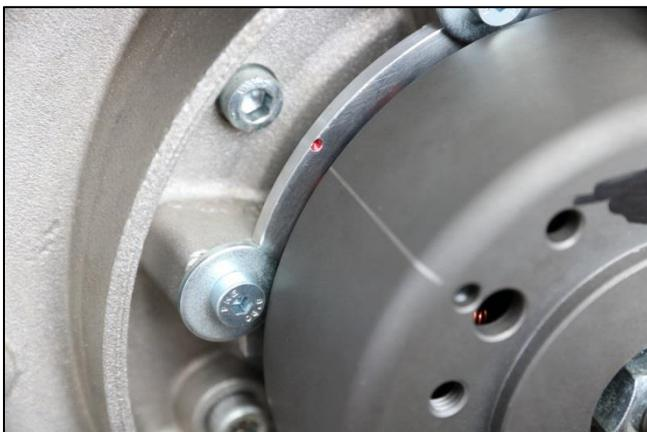
Abbildung 4 – TDC mark for pre-adjusting the Ignition
